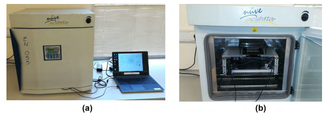
FIGURE 21. Incu-Stream test stage in a non-CO 2 and dry incubator: (a) Cabling and location of host computer; (b) inner view of the incubator with lid open.
