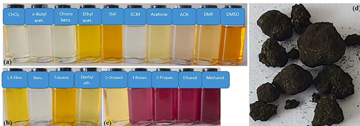
Fig. 1. Solutions of 4odna in different solvents: (a) polar-aprotic; (b) non-polar; (c), polar-protic, and (d) a sample of the solid compound. In each group, the solutions are ordered by increasing dielectric constant ( \epsilon ) of the solvent.
