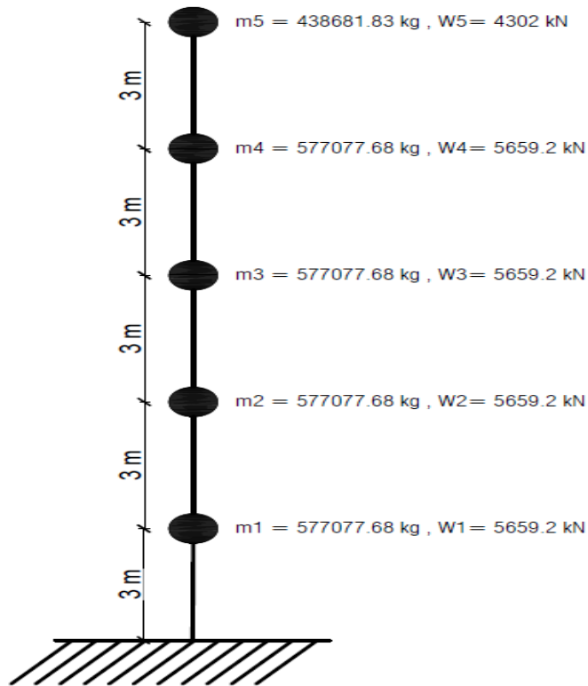
Figure 5.2 : Story Masses According to TEC2007
