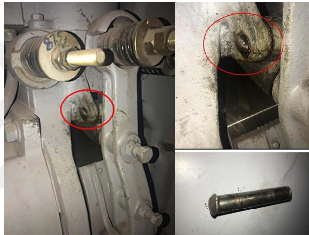
Figure 2.5: The motor brake shaft pin without safety clip
