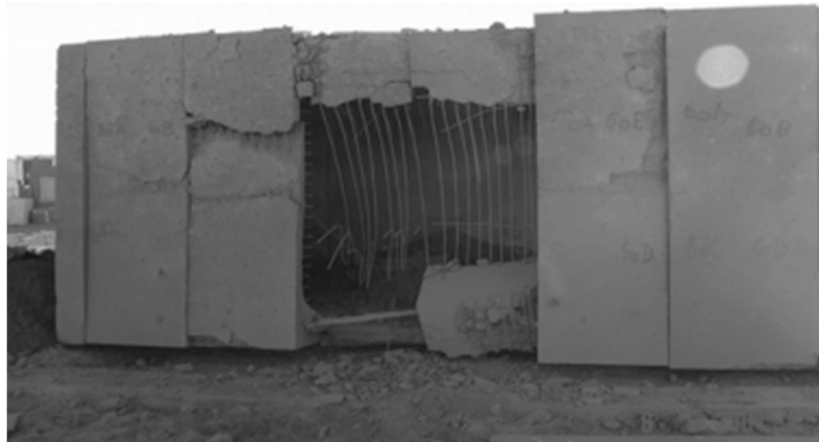
Figure 2.13: Breaching failure due to a close-in explosion of 6000kg TNT equivalent.[3]
