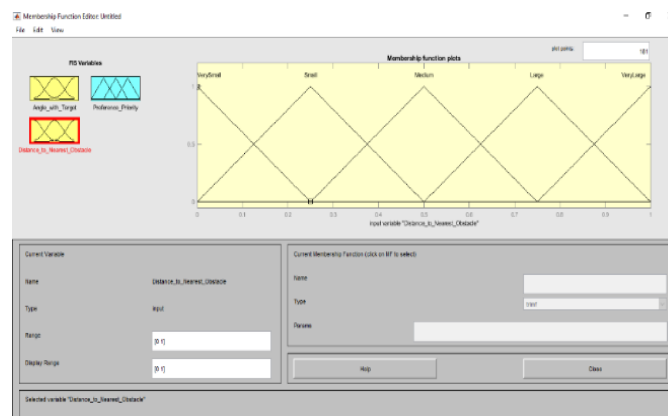
Figure 5.9- Distance_to_Nearest_Obstacle Input Membership Functions
