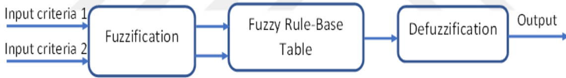
Figure 5.7- The Illustration of the Suggested Fuzzy Logic for Mobile Robot Path Planning
