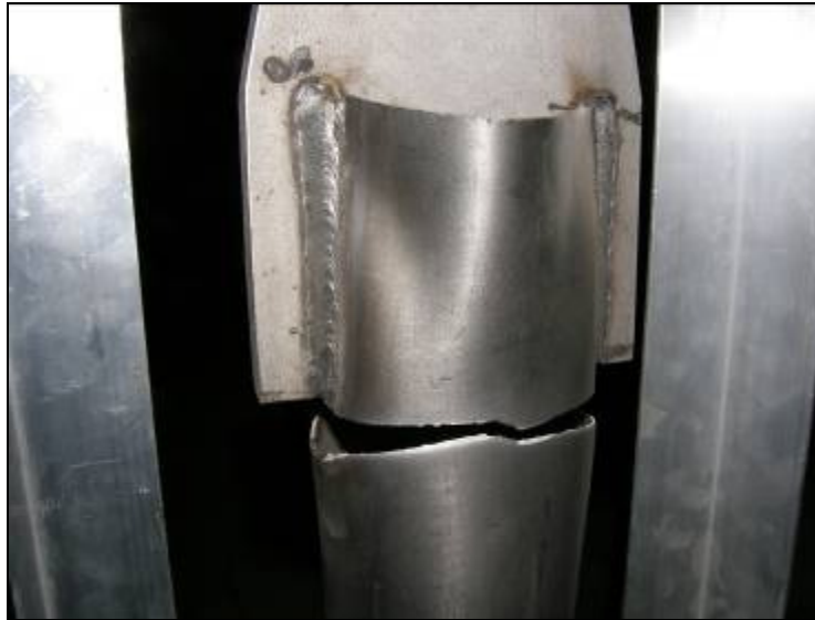
Figure 5 Typical failure mode observed in all the test specimens
