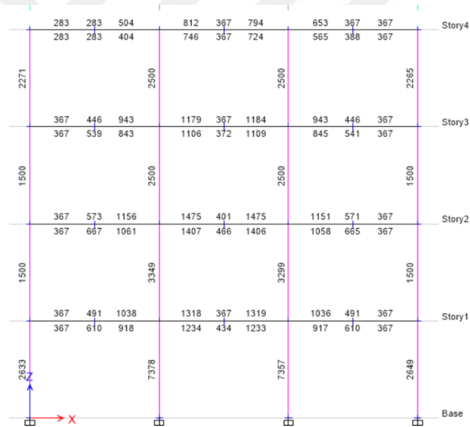
Figure 4.28: Steel Area for the Columns and Beams.
