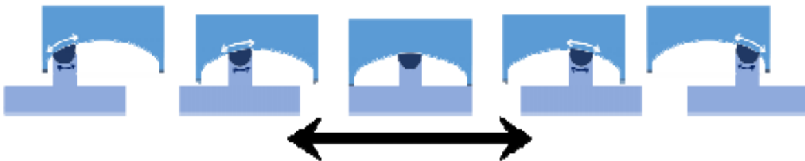
Figure 2.10: Behaviour of FPS during an Earthquake [43]
