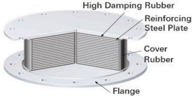
Figure 2.5: High-Damping Rubber Bearing [24]
