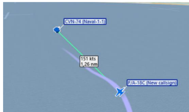
Figure 7. Tacview measurement of system maximum guidance distance in sunrise conditions.
