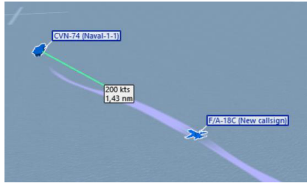
Figure 9. Tacview measurement of system maximum guidance distance in sunset conditions.
