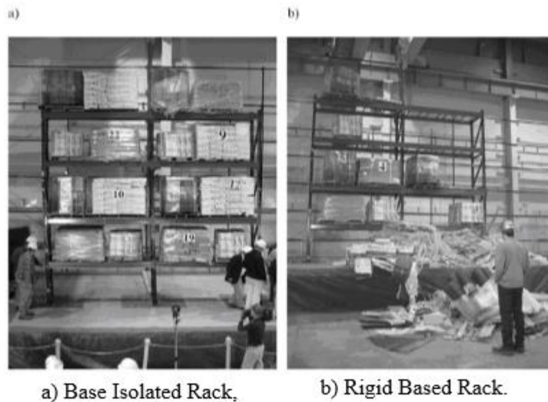
Figure 12: Base isolated and rigid based racks under Tri-Axial Seismic Excitations experiment [11].
