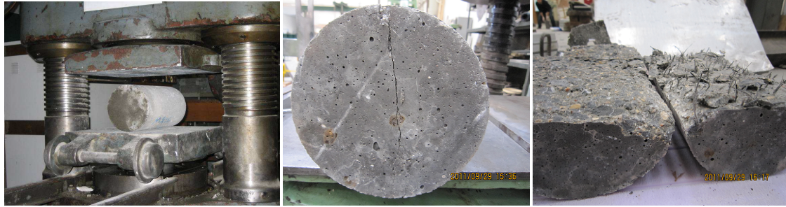
Figure 9- The device of doing Brazilian tensile test and specimen fracture and removing fibers from concrete
