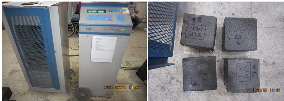
Figure 7- The system of testing compressive strength and cubic concrete specimen
