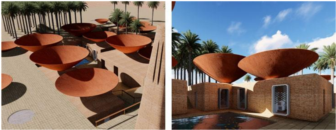
Şekil 5.5 Concave Roof System (URL-21) (URL-22)
